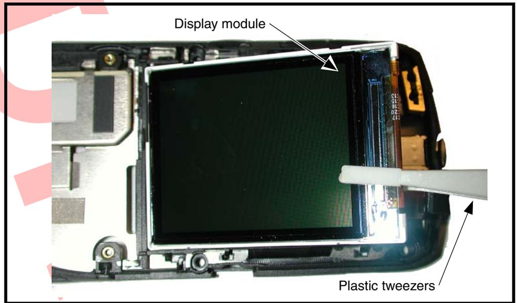
**Figure 21. Removing the Display Module**
