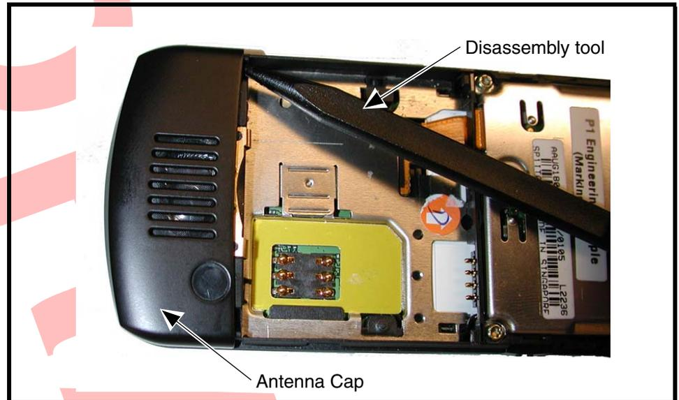
Figure 7. Removing the Antenna Cap
