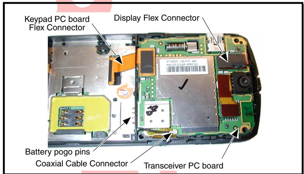
**Figure 10. Removing the Transceiver PC Board Connectors**
