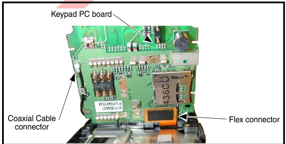
Figure 18. Removing the Keypad PC Board Flex Connector
